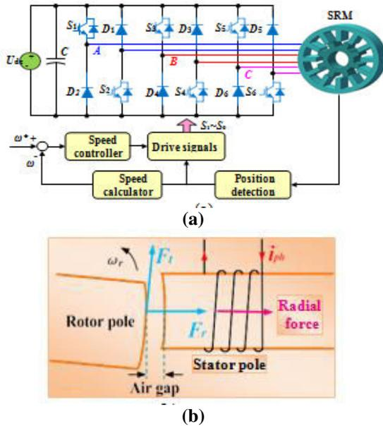
**Fig. 2. SRM drive and attraction force. (a) Three-phase SRM drive. (b) Attraction force produced by stator and rotor poles.**
