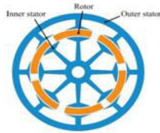
**Figure 4. Double stator SRM structure [32], [33].**
