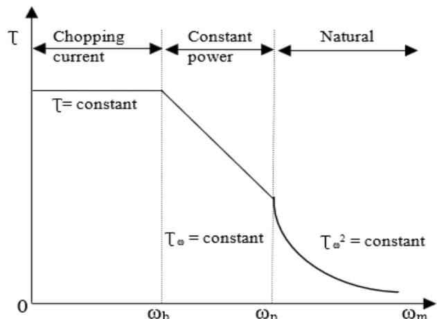
**Figure.8. Torque speed characteristic of SRM**
