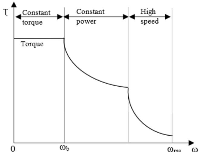
**Figure.7. Torque speed characteristics of PMSM**
