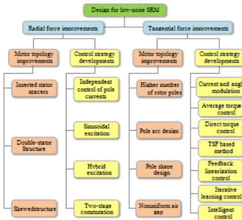
Figure.1. Classification of possible developments for low-noise SRM drives.
