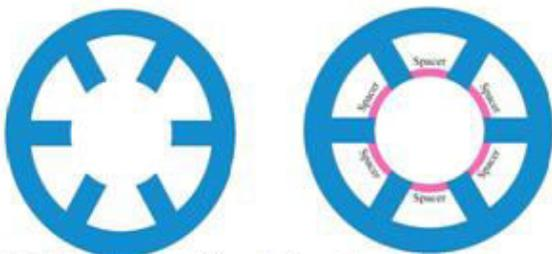
**Figure 3. Stator structure with and without structural stator spacers (a) Conventional stator. (b) Developed stator [28].**
