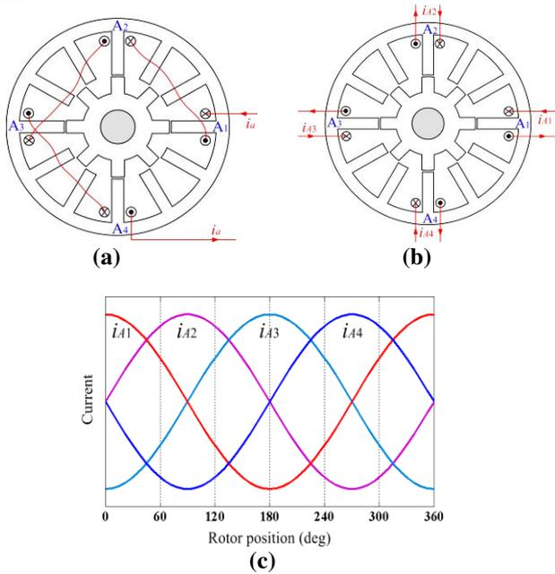
**Figure.6. Independently controlled pole currents. (a) Series pole windings. (b) Independent pole windings [19]. (c) Sinusoidal excitations [20].**
