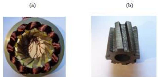
**Figure 5. Skewed motor structure [36]. (a) Skewed stator. (b) Skewed rotor.**
