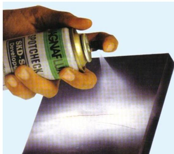
Figure.4. Application of Developer
