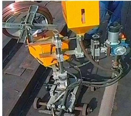
The process is normally limited to the flat or horizontal-fillet welding positions (although horizontal groove position welds have been done with a special arrangement to support the flux).
