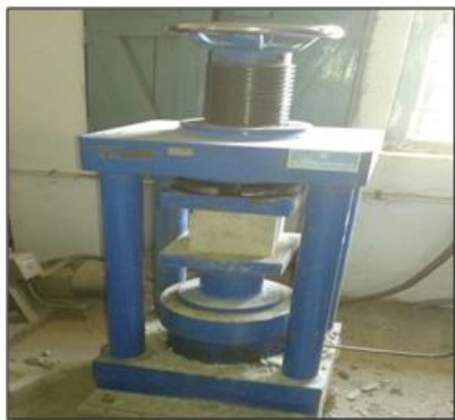
Figure.5. Compressive strength testing
