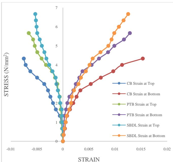
**Figure. 5. Stress v/s Strain for CB, PTB and SBDL**
