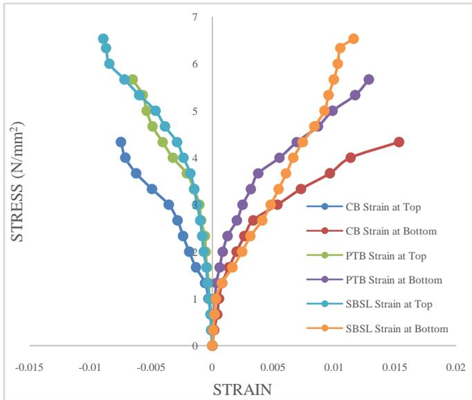
**Figure.4. Stress v/s Strain for CB, PTB and SBSL**
