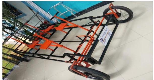
FIGURE 5.5.1 Final Assembly of Rowing Human Powered Car
