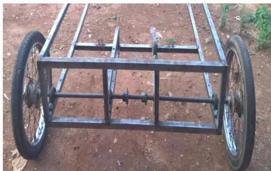
FIGURE 5.3.1 Rear axle Assembly
