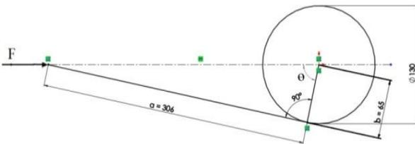
FIGURE 4.1.2 Determination of Torque at the crankshaft
