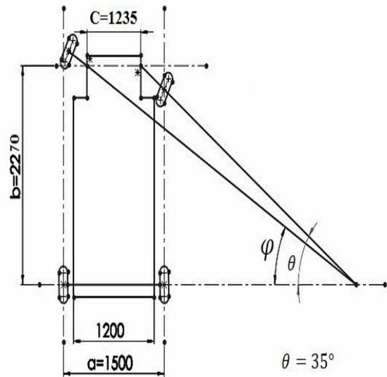
FIGURE 4.3.1 Determination of Turning radius
