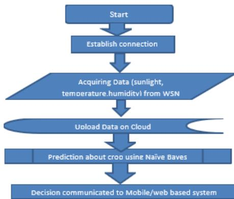
Step1: Connection will be established between the IoT device and Cloud.
