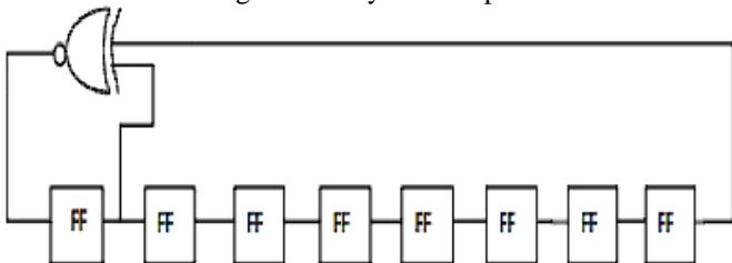
**Figure .2. An example of the modified LFSR TPG**
