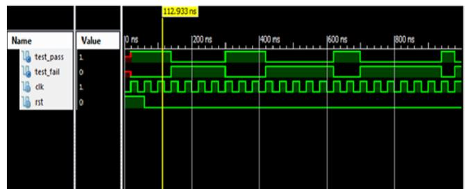
**Figure.4. Existing method Simulation BIST\_LFSR**
