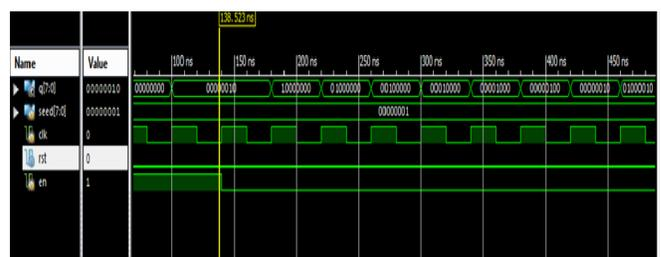
**Figure.5. Proposed method Simulation BIST\_LP-LFSR**
