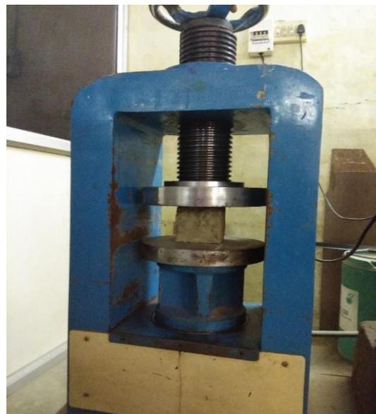
**Figure.4. Compressive Testing Machine**
