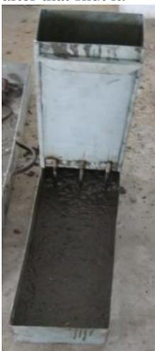
**Figure.2. L Box Test**
