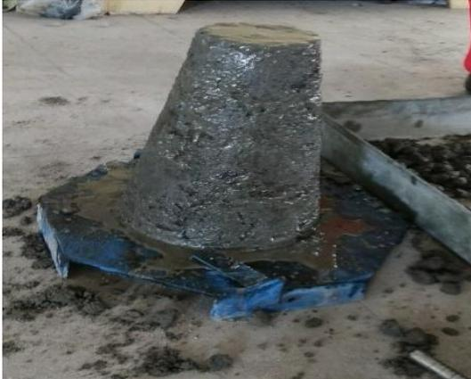
**Figure.1. Slump Cone Test**
