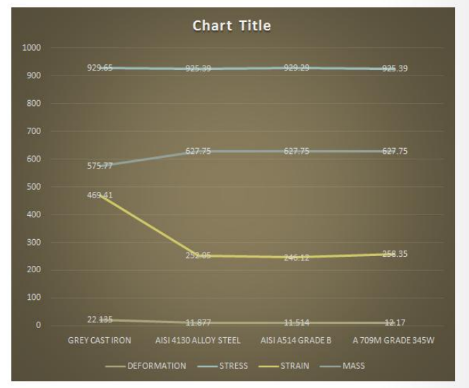
Graph.1. Comparative analysis of structural steel chassis, other alloy steels & composite materials
