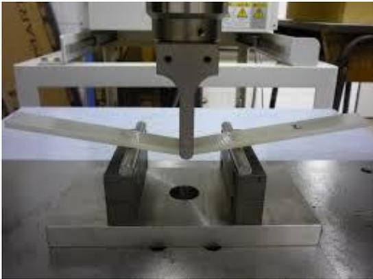
Figure.2. Three point bend test apparatus
