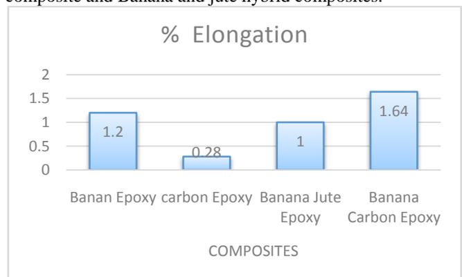
Figure.4. Effect of fiber loading on Percentage of elongation
