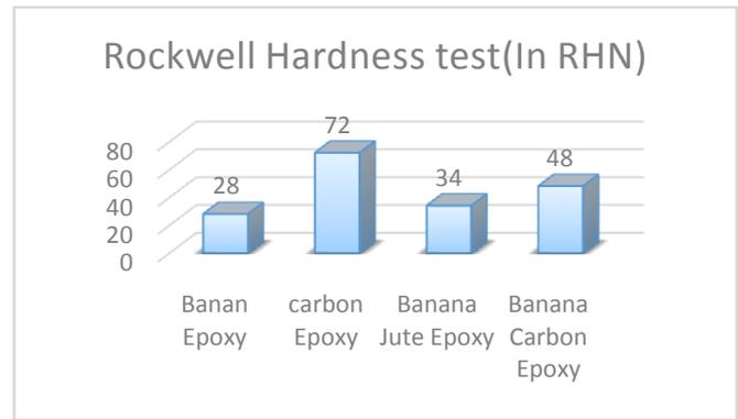
Figure.7. Rockwell Hardness test
