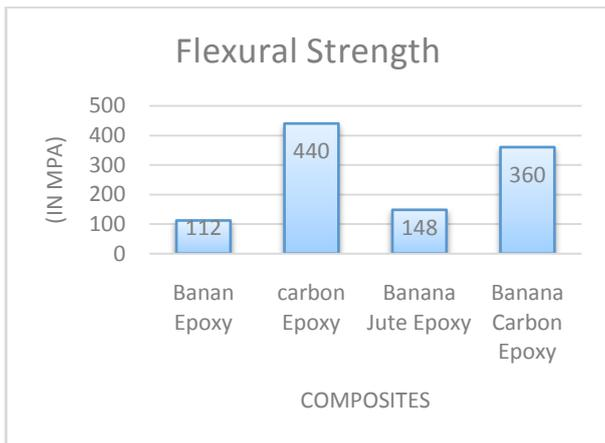
Figure.5. Effect of fiber loading on Flexural Strength
