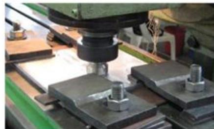
Figure.3. Experimental FSW
