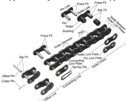
Connecting Link: This is the ordinary type of connecting link. The pin and link plate are slip fit in the connecting link for ease of assembly. This type of connecting link is 20. Percent lower in fatigue strength than the chain itself. There are also some special connecting links which have the same strength as the chain itself.
