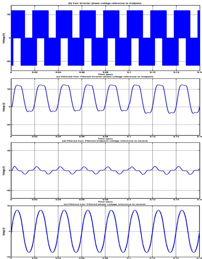
**Figure. 5.2.** Simulated inverter waveforms. (a) Vab-Phase to phase inverter voltage (b) Vao- Inverter phase voltage reference to midpoint. (c) Filtered Von- Filtered inverter phase voltage reference to midpoint. (d) Filtered Von- Filtered midpoint voltage reference to neutral. (e) Filtered Van- Filtered phase voltage reference to neutral.
