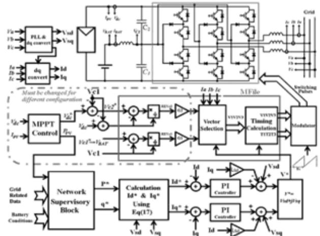
Figure. 5.7: Control system diagram to integrate PV and battery storage.
