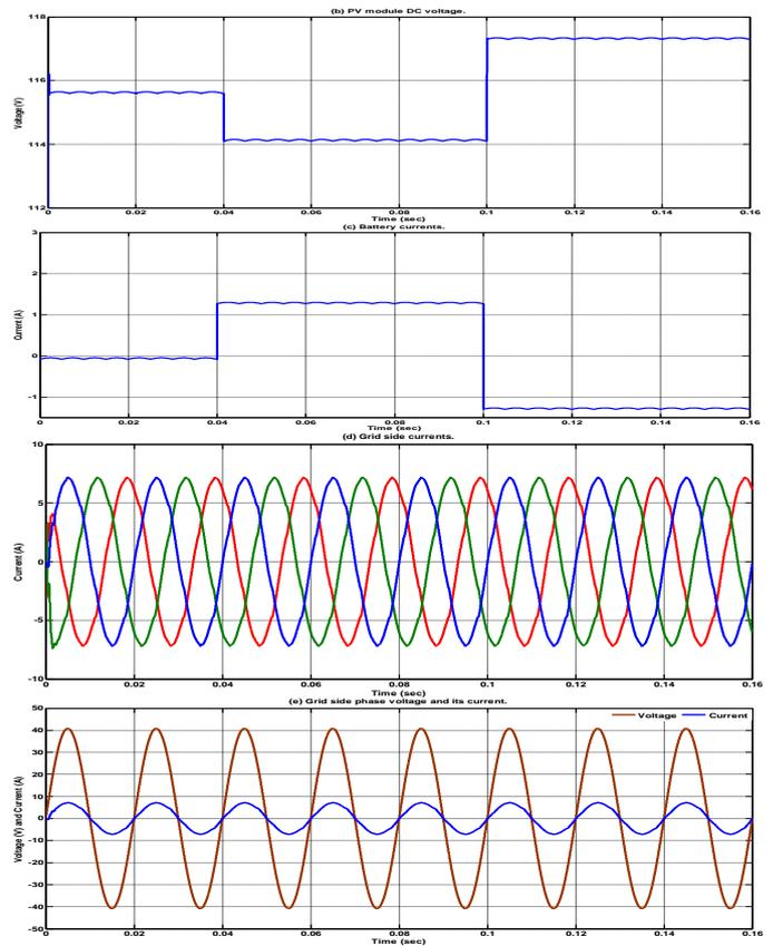
**Figure.5.3.** Simulated results for the second scenario. (a) Active power injected to the grid. (b) PV module DC voltage. (c) Battery currents. (d) Grid side currents. (e) Grid side phase voltage and its current.
