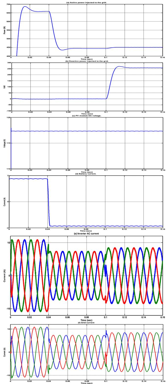
**Figure .5.1. Simulated results for the first scenario (a) Active power injected to the grid. (b) Reactive power injected to the grid. (c) PV module DC voltage. (d) Battery current. (e) Grid current.**
