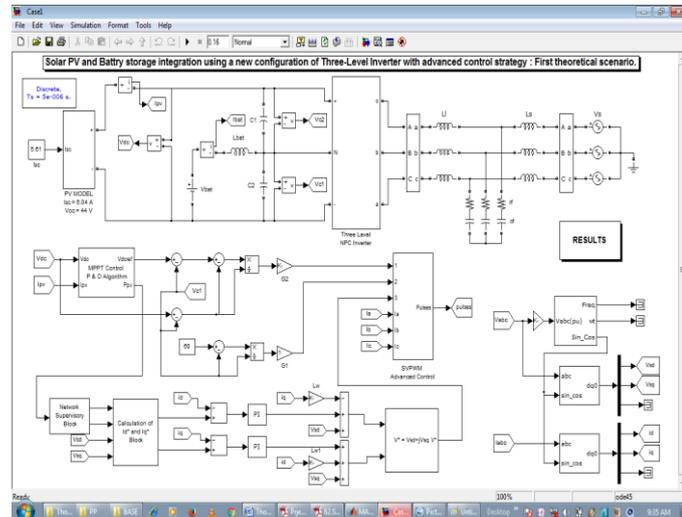
**Figure.4.2: MATLAB / Simulink model of solar PV and battery storage integration using NPC inverter.**
