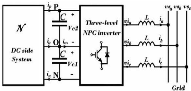
Figure. 2.1: General diagram of a grid connected three-wire three-level inverter. [1]
