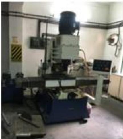
**Figure.1. Friction stir welding Equipment**
