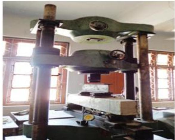
Figure.1. Complete test set up in UTM
