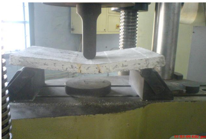
5.1 Testing of ferrocement panel
