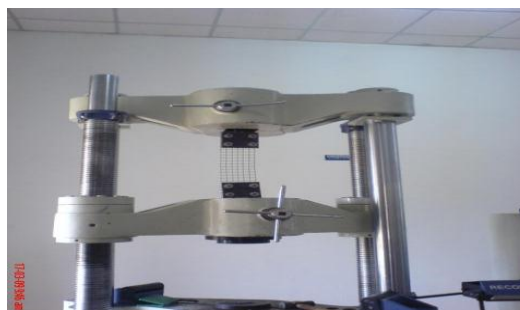
Fig 4.1 Testing of wire mesh
