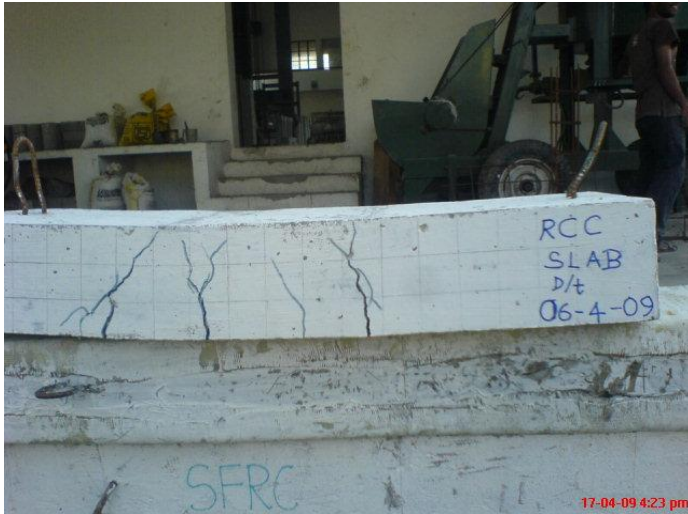
5.3 RCC Slab after Testing
