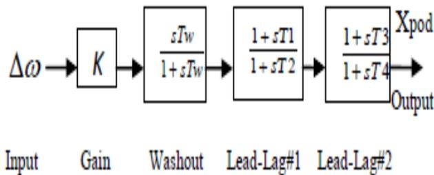
Figure.2. Block Diagram of Pod Controller
