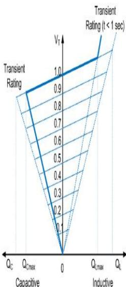
Figure.8. Operating characteristics of the STATCOM
