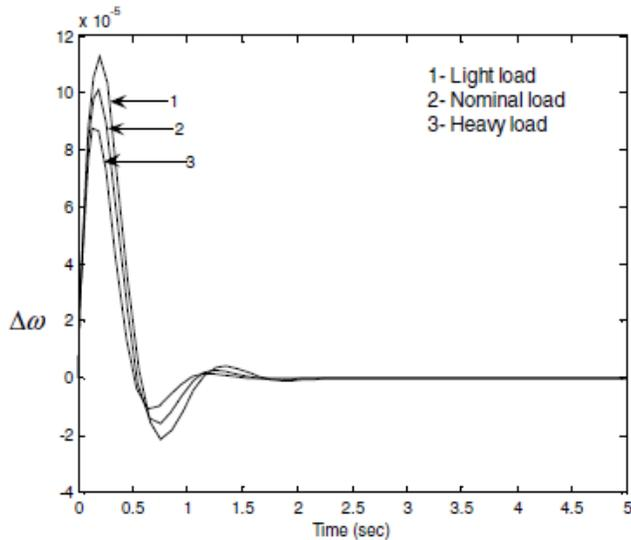
**Figure.11. 3 Dynamic response for w with the IPFC based damping controller for different loading conditions.**
