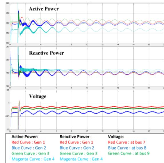
**Figure.12. 2:** the system with STATCOM without POD function, connected at bus 7 when a three phase to ground fault applied at  $t = 1$  s and 0.05 s.
