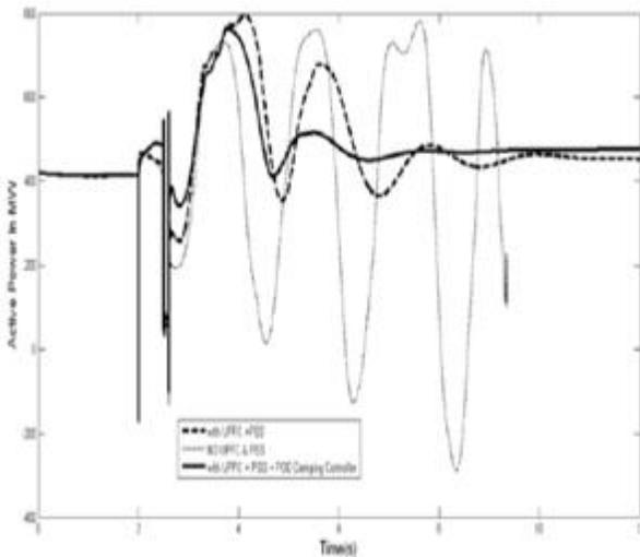
Figure.10. 3: Active power in MW with UPFC+POD+PSS and without PSS and UPFC
