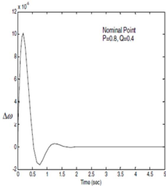
**Figure.11. 2: Dynamic response for DW with the IPFC based damping controller**
