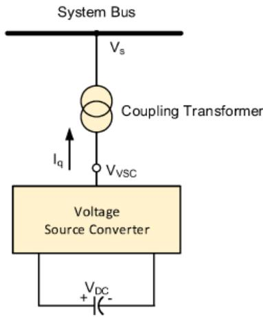
Figure.7. Schematic of the STATCOM.
