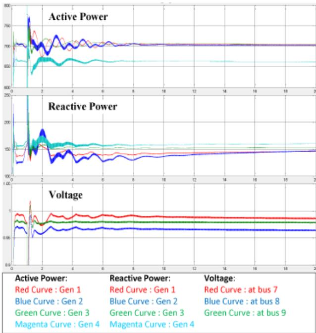
**Figure 12. 3: The system with STATCOM and POD function, connected at bus7 when a three phase to ground fault applied at  $t = 1$  and  $fct 0.05$  s.**
