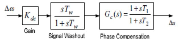
Figure.6. Structure of IPFC based damping controller
