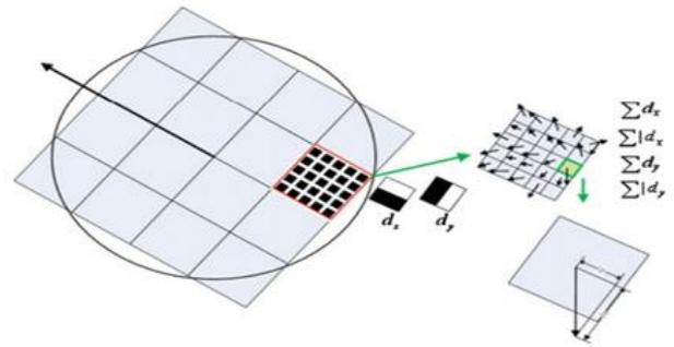
Figure.5.D.2 dividing the interest region into  $4 \times 4$  sub-regions for computing the SURF descriptor
