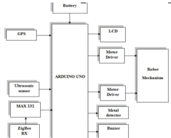
**Figure.1. Transmission section of the robot**
