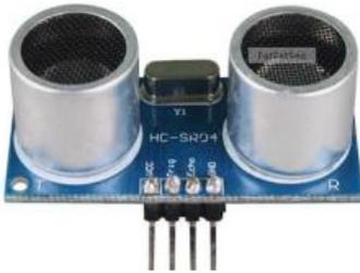
**Figure.4. Ultrasonic sensor**
