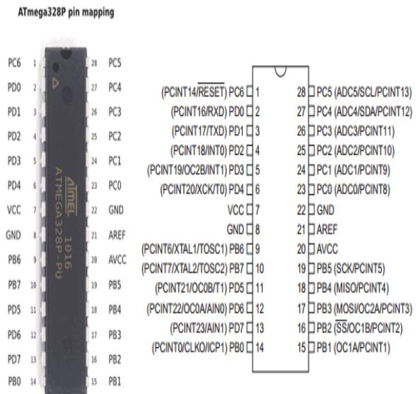
**Figure.3. Arduino Microcontroller**
