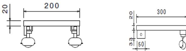
Figure.11. 2D view of wheeled robot
