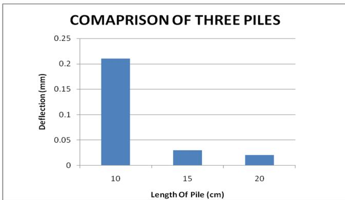
**Figure.6. Comparison of Three Piles of Different Lengths**
