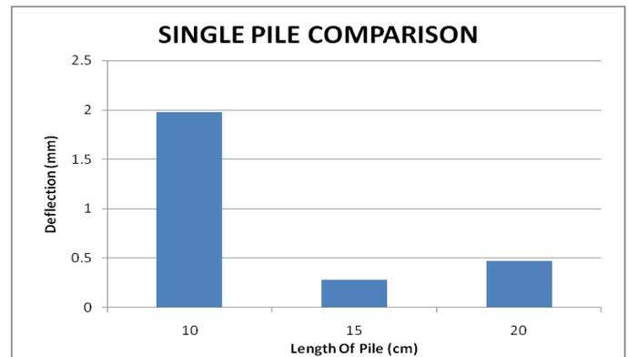
Figure.4. Comparison of Single Piles Of Different Lengths
