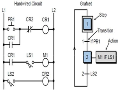
**Figure.3.4 Hardwired logic circuit and its grafset representation**
