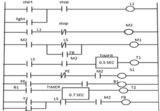
**Figure 4.2 Ladder diagram for bottle filling system**
