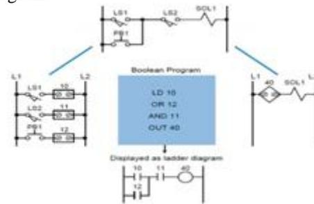
**Figure. 3.2 Hardwired logic circuit and its Boolean expression**
