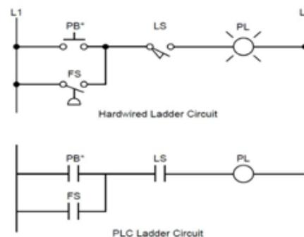
**Figure 3.3 Hardwired logic circuit and its PLC ladder diagram representation**
