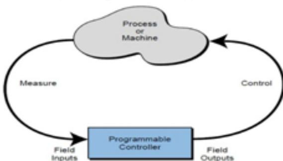
Figure.1. PLC conceptual application diagram
