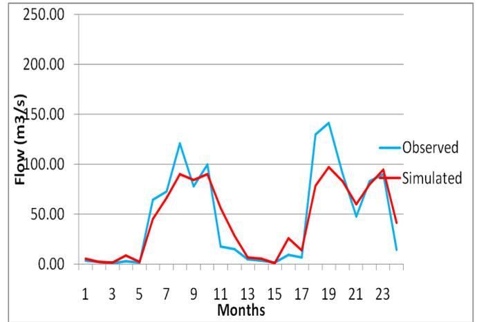
**Figure.2. Observed and simulated Flow before Calibration**
