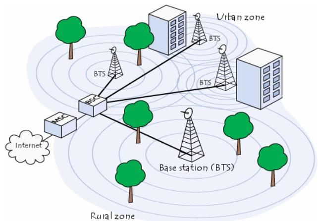
**Figure.5. Architecture of GSM network**
