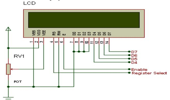
Figure.8. Block diagram of LCD
