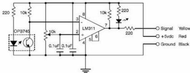
**Figure.10. schematic diagram for single pair of infrared transmitter and receiver**
