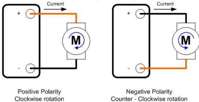
Figure.7. DC Motor with clock and anti clockwise direction
