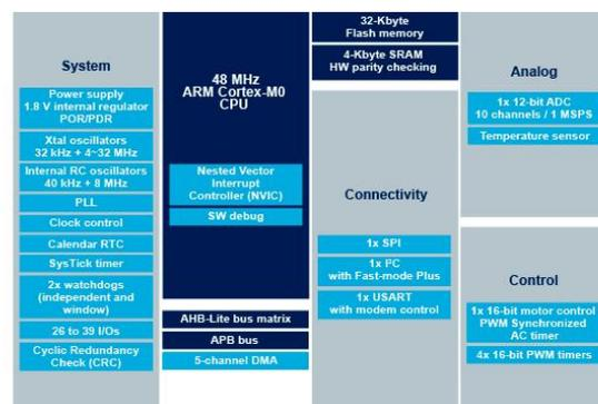
**Figure.2. Block Diagram of Micro Controller**
