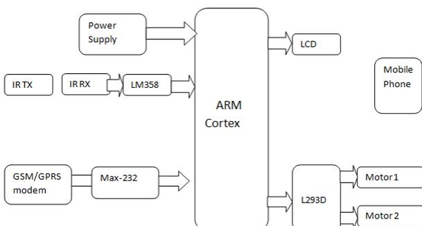
**Figure.1. Block Diagram of Automatic Detection of Squats in Railway Track**
