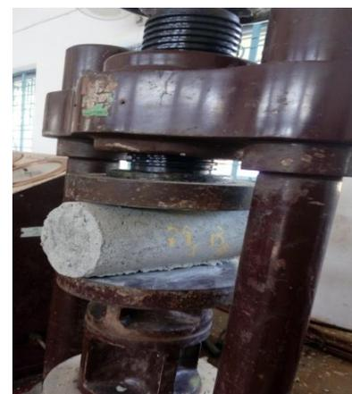
**Following Figure.5. show the photographic view of split tensile strength test and failure of specimen.**
