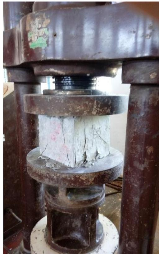
**Figure.4. show the photographic view of compressive strength test and failure of specimen.**
