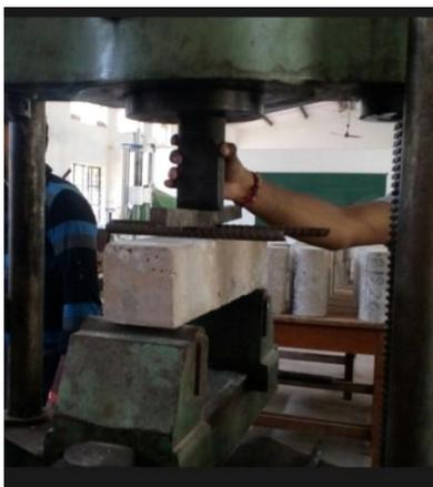
**Figure.6. Flexural strength test.**
