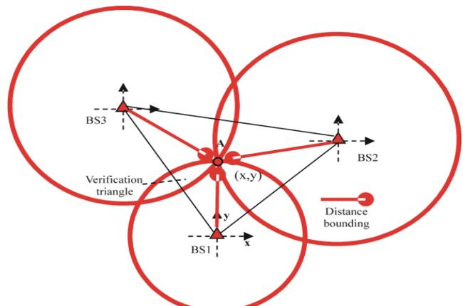
Fig.4. Trilateration method used in Wifi Positioning.
