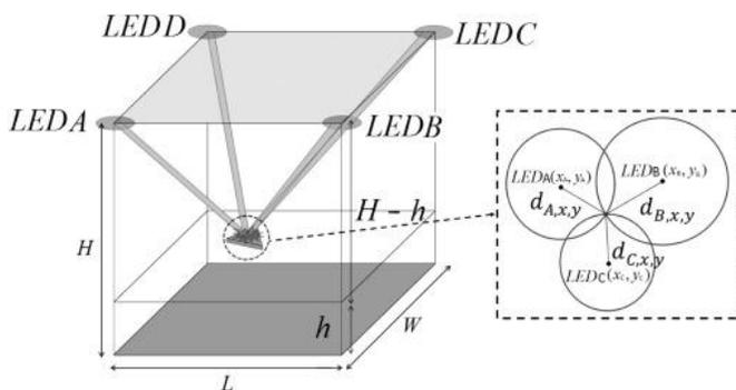
Fig.3. Determining position using VLC
