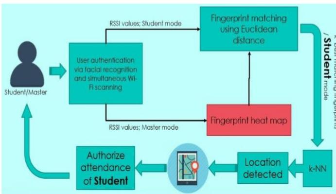
Fig.8. Working Of Student Monitoring System Using Wifi
