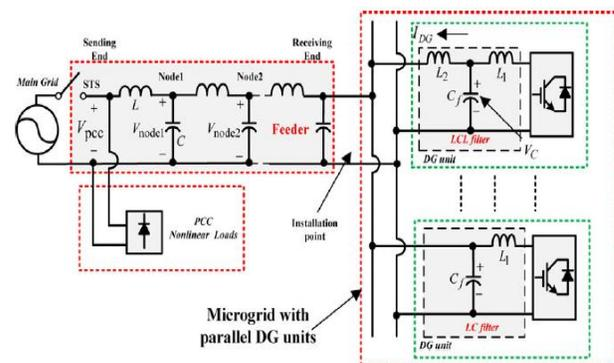
**Figure.1. Circuit Diagram**
