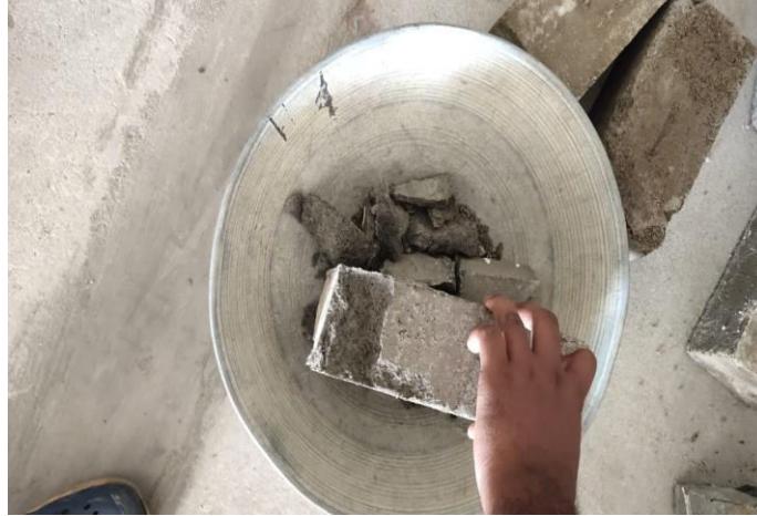
After the compression test
