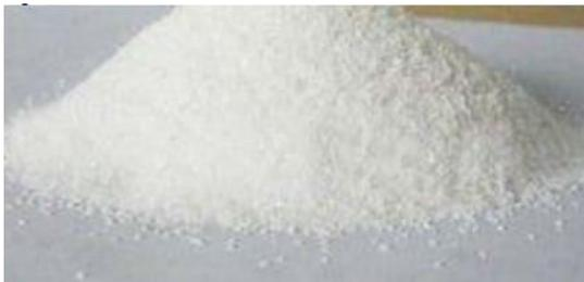
Figure 2.2 Aluminium oxide powder (Alumina Powder, Al<sub>2</sub>O<sub>3</sub>)
