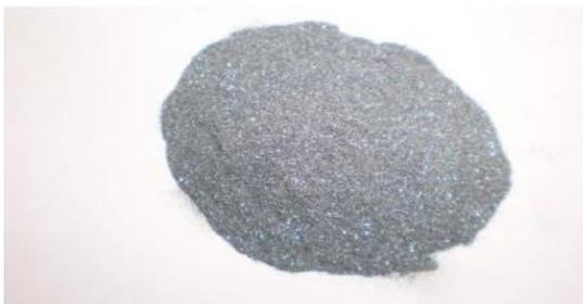
Figure-2.3 Silicon Carbide (SiC)
