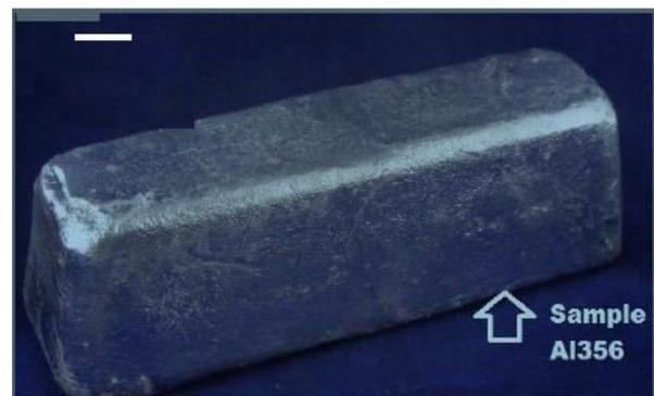
Figure.2.1. Aluminum Alloy Al356 sample
