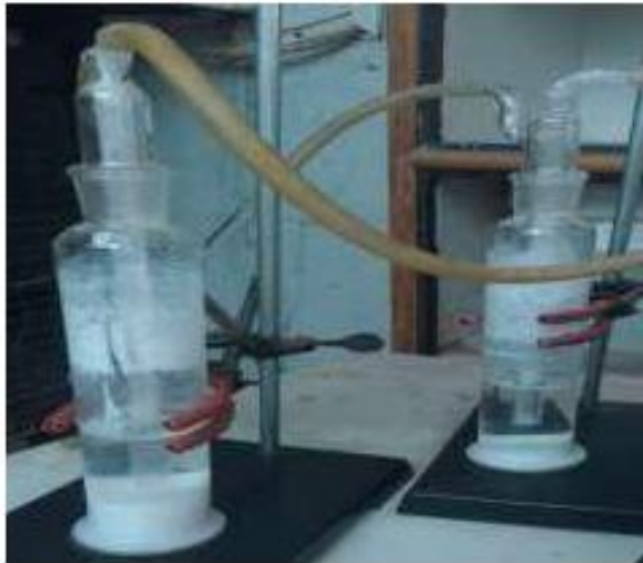
Figure.3. Ba (OH) 2 precipitate of Contain 1 and Container 2 The amount of CO 2 evolved was calculated by
