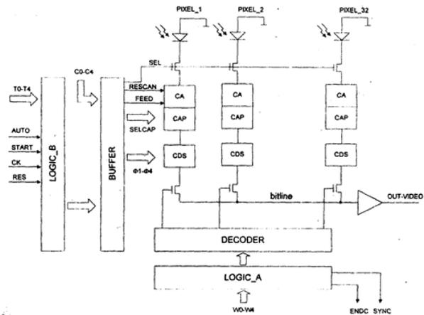
Figure6 Block diagram of the 32-pixel prototype array.
