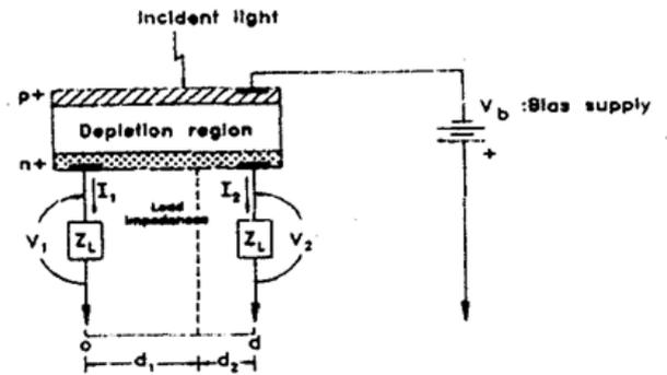
**Figure3 Basic structure of a single-axis lateral effect photodiode**
