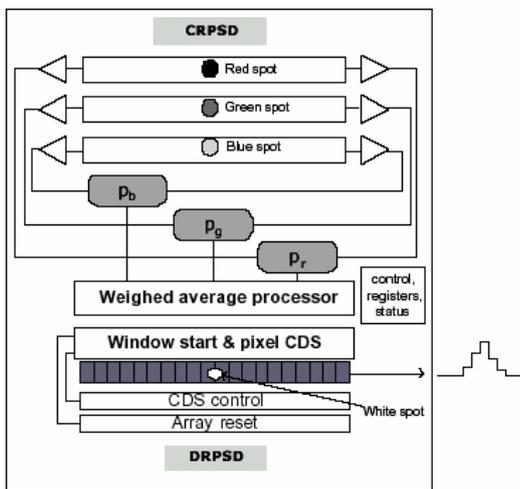
Figure5 The proposed architecture for the colorange chip
