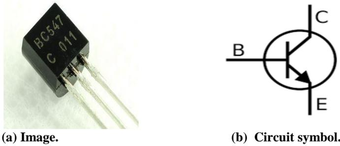
**Figure.4. Image and circuit symbol of a transistor.**
