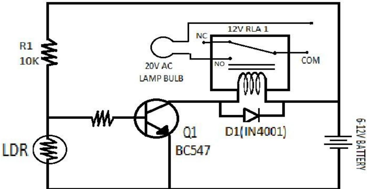
Figure .9. Circuit layout of LDR based dark detector.
