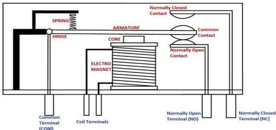
Figure.12. Internal structure of a relay.
