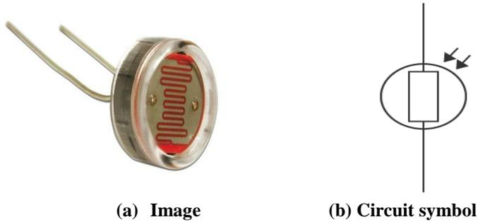
**Figure.3. Image and circuit symbol of an LDR.**
