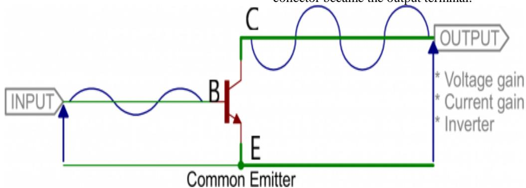
Figure .11. Amplified output signal in common emitter configuration.
