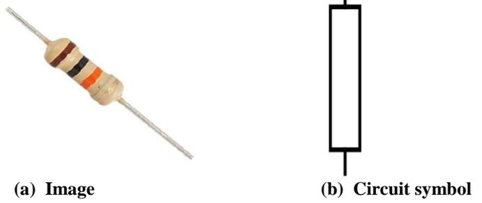
**Figure 5: Image and circuit symbol of a 10kΩ resistor.**
