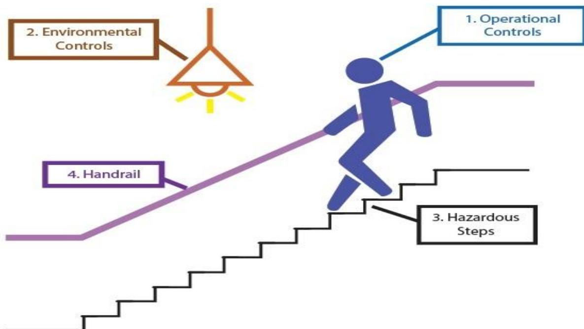
Figure.1. Dependent elements on safer stairs and steps.
