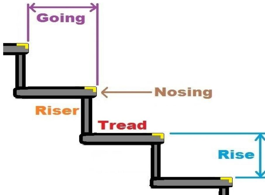
Figure.2. Parts of a stair.
