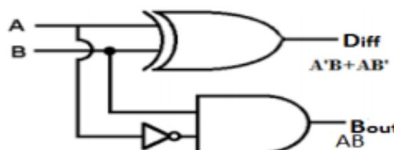
Figure.2. Gate Level 1 bit Conventional Half Subtractor.
