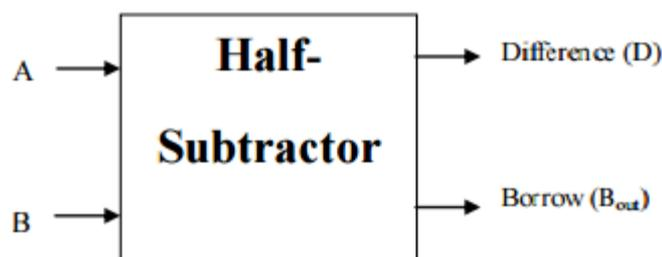
Figure.1. Logic Symbol of half Subtractor
