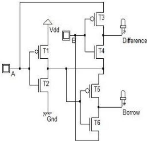
**Figure.3. Circuit diagram of Conventional Half Subtractor**
