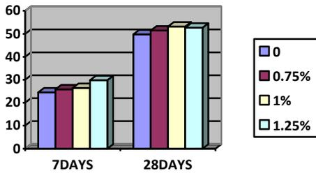
**Figure. 5 Compressive strength of steel fibre concrete at a distance of d/2 from the bottom (d=total depth of specimen)**
