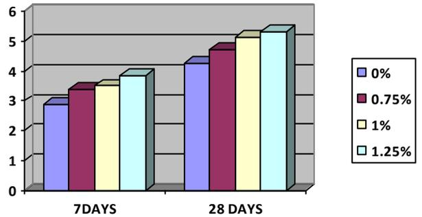
**Figure.7.Split tensile strength of steel fibre concrete at a distance of d/2 from the bottom**
