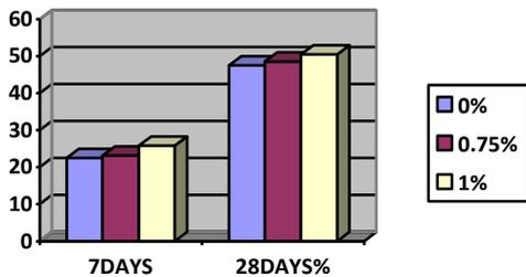
**Figure. 5 Compressive strength of steel fibre concrete at a distance of d/3 from the bottom (d=total depth of specimen)**
