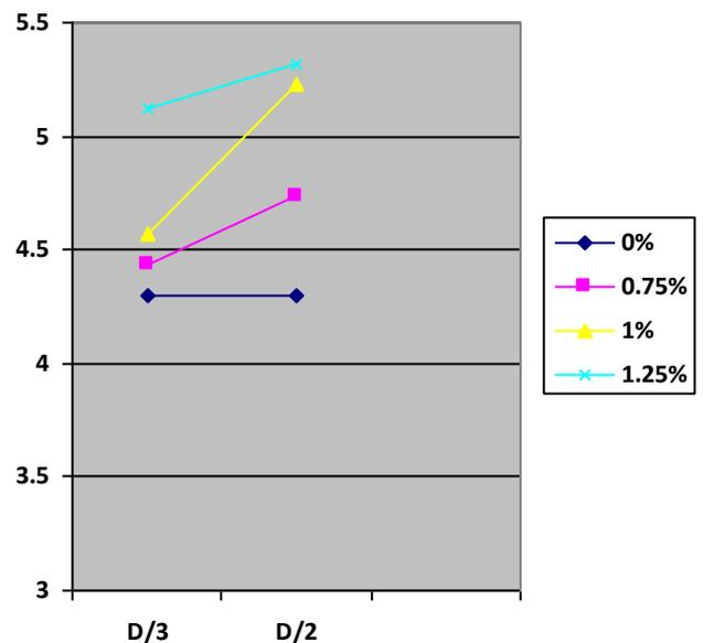
**Figure.8. Flexural strength of SFRC with 0%, 0.75%, 1%, 1.25% fibres M50 grade**
