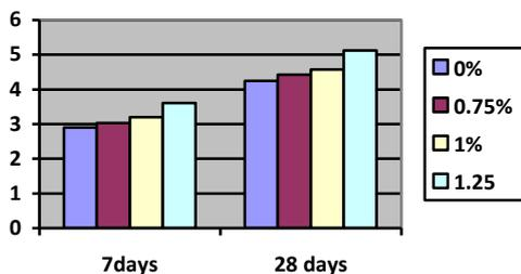
**Figure.6. Split tensile strength of steel fibre concrete at a distance of d/3 from the bottom**
