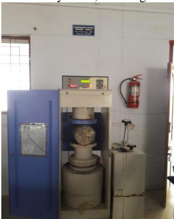
Figure. 2. "Testing of Split tensile strength test specimen"
