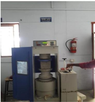
Figure. 1. "Testing of compressive strength test specimen"
