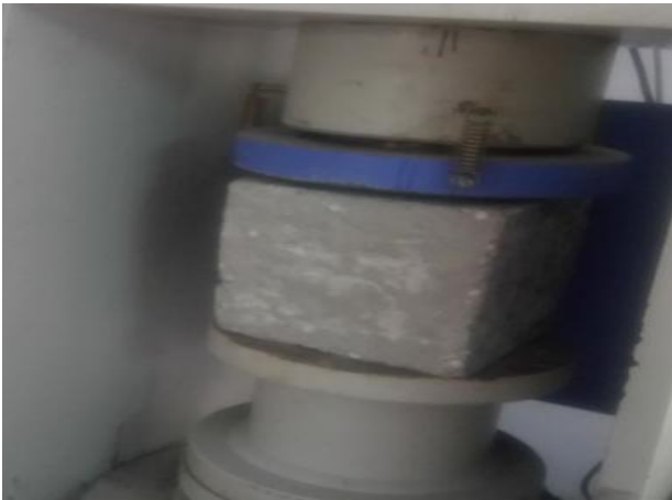
Fig: 3 Compressive strength test
