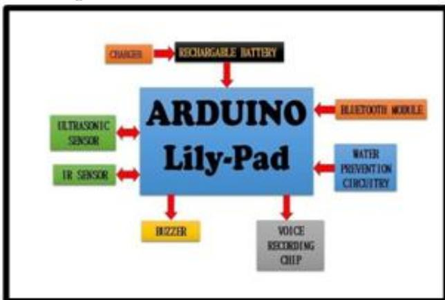
**Figure.9. Block Diagram of Cane Module**
