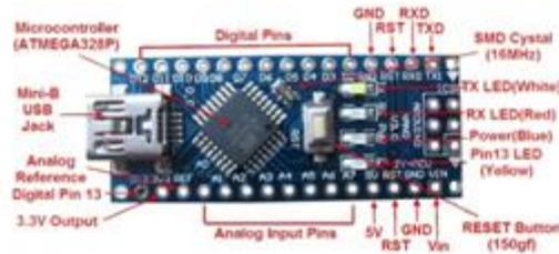
**Figure.8. Parts of Arduino Nano Difference between uno and nano**
