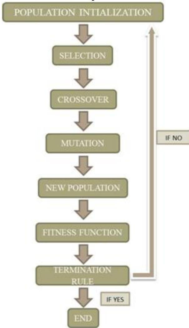
Figure. 1. Genetic algorithm flow diagram
