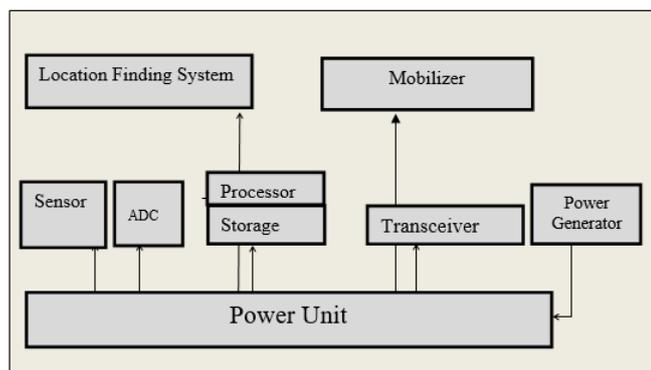
Fig. 1 Components of Wireless sensor node [1]
