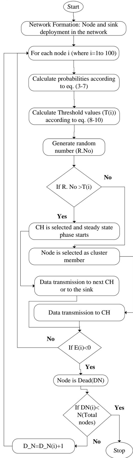
Fig. 5 Flow chart for CH selection in proposed work
