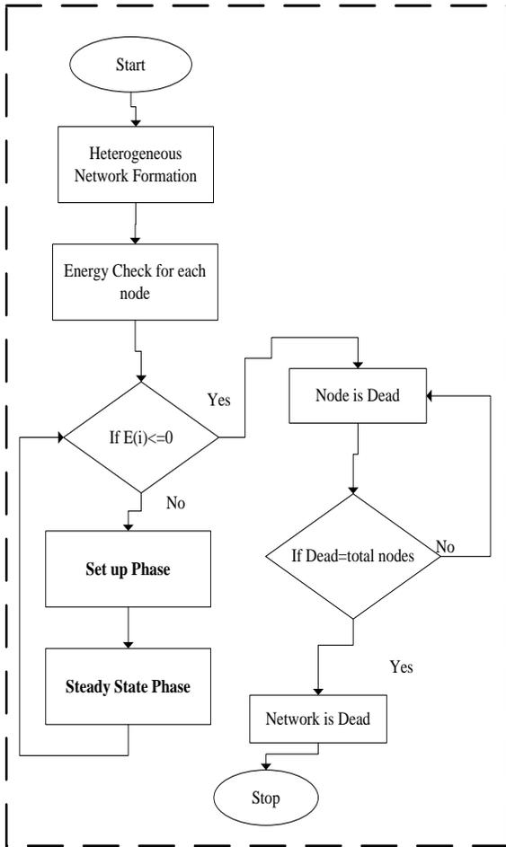
Fig. 4. Flow chart for the network scenarios in heterogeneous protocols
