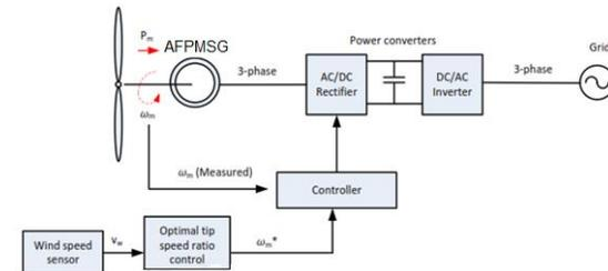
Figure.10. Tip speed ratio control scheme
