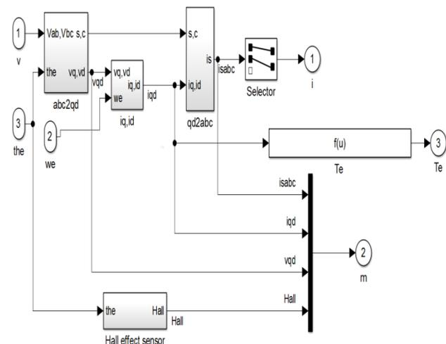
Figure.7. Dynamic model of the considered AFPMSG.
