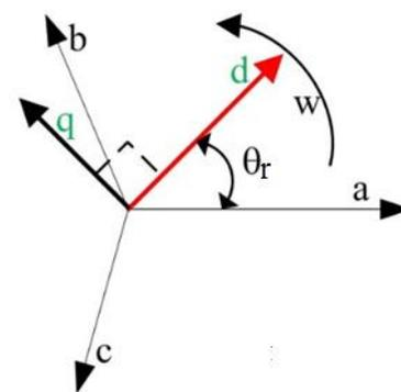
Figure.5. Park transform for AFPMSG generators.
