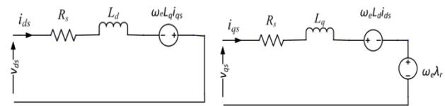
Figure.6. The dq-axes equivalent circuits of a AFPMSG in (consumer/load) notation
