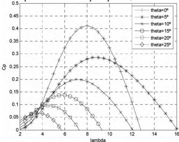
Figure.3. Coefficient of power ( $C_p$ ) versus Tip-speed ratio ( $\lambda$ )
