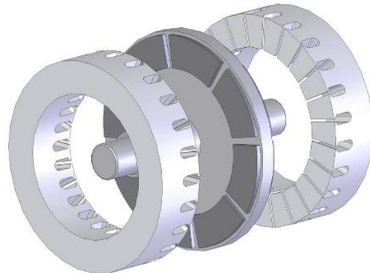
Figure.2.Magnetic circuit parts of an AFPMSG with one rotor-two-stators.
