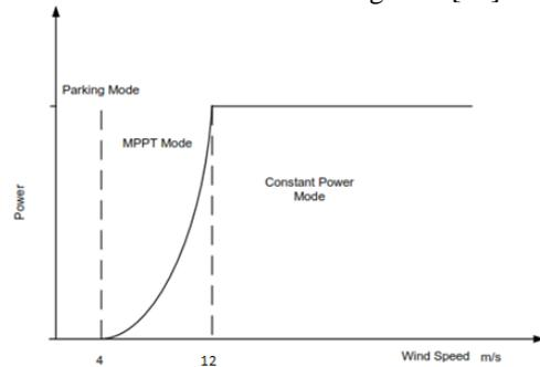
Figure.9. Wind turbine power-speed characteristic for the specific wind turbine
