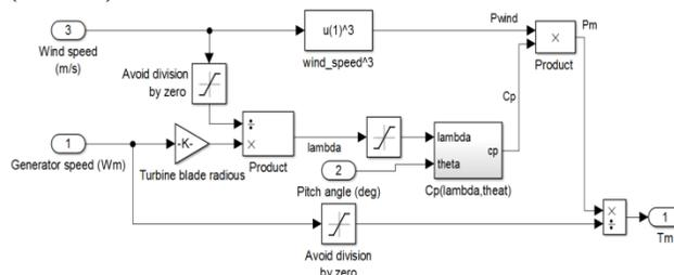
Figure.4. Wind turbine Simulink model.
