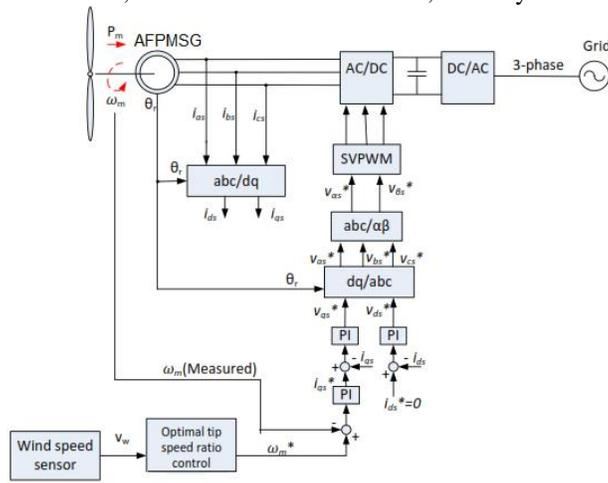
**Figure.12. Generator-side control scheme**
