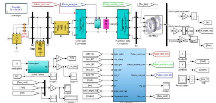
**Figure.13. Control diagram of the system**
