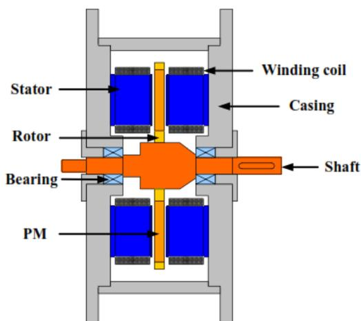
Figure.1. Cross section views of the AFPMSG
