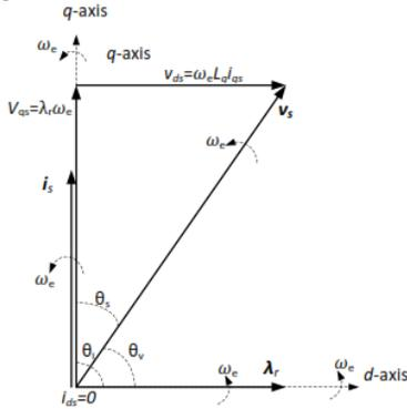
**Figure.11. Phasor diagram of the FOC**
