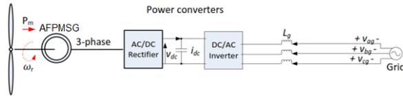
Figure.8. Direct-drive AFPMSG system
