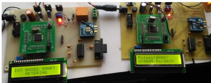
Figure.4. output of meter 1 is being sensed and transmitted. Data is locally displayed on the lcd panel
