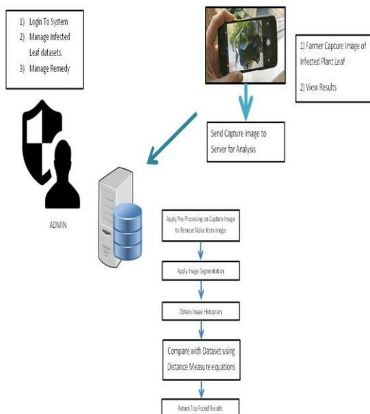
**Figure.1. Block Diagram of System**
