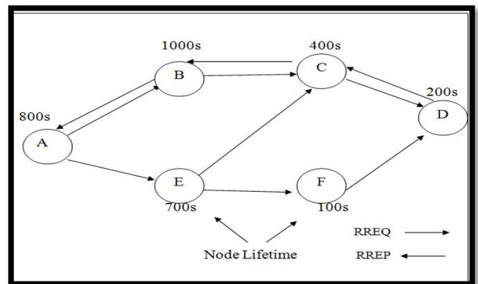
Figure.2. Routing discovery and maintenance for ABR
