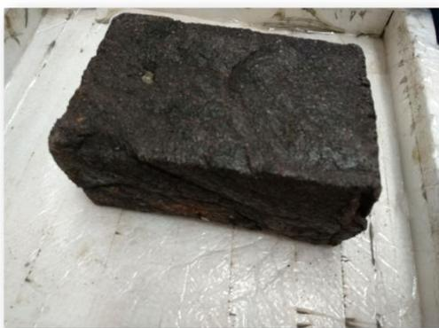
**Figure. 1. Soil-plastic brick casted**
