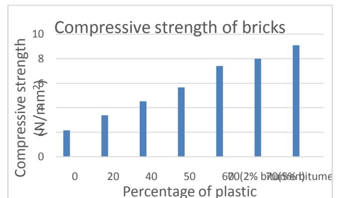
**Figure.3. Bar graph showing the results of compressive strength**
