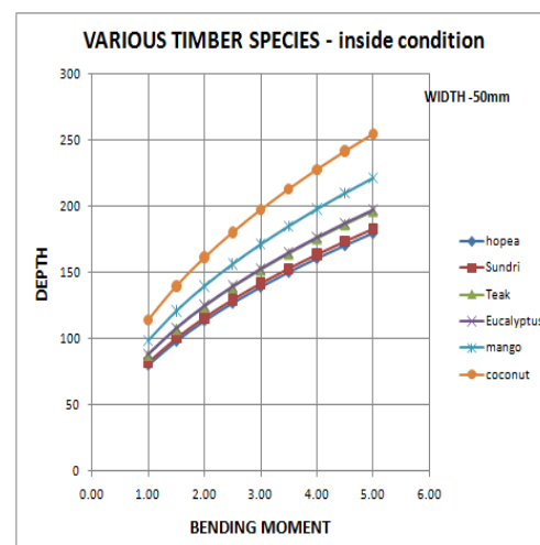
Graph.5. Bending Moment Vs depth for inside condition for 50mm width
