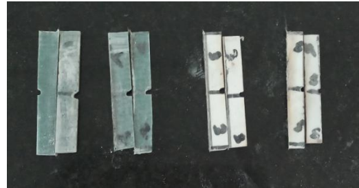
Figure.1. Tensile, Flexural and Impact test Specimens
