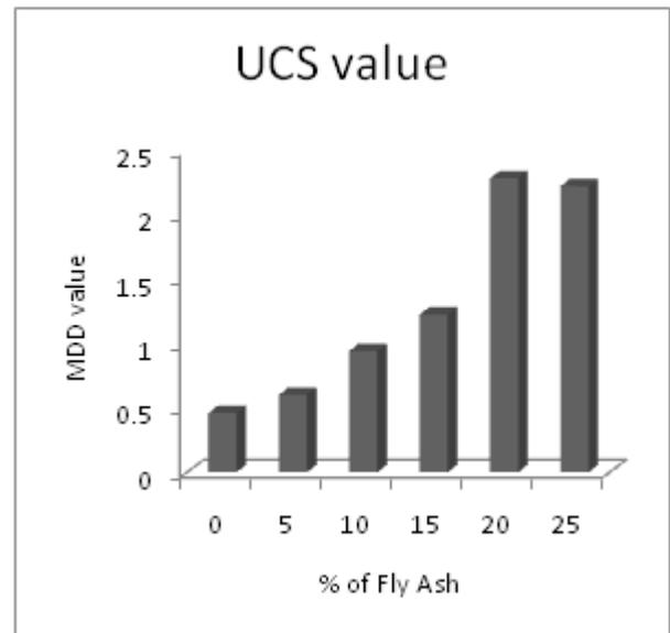
Figure.8. Effect of Fly Ash on UCS
