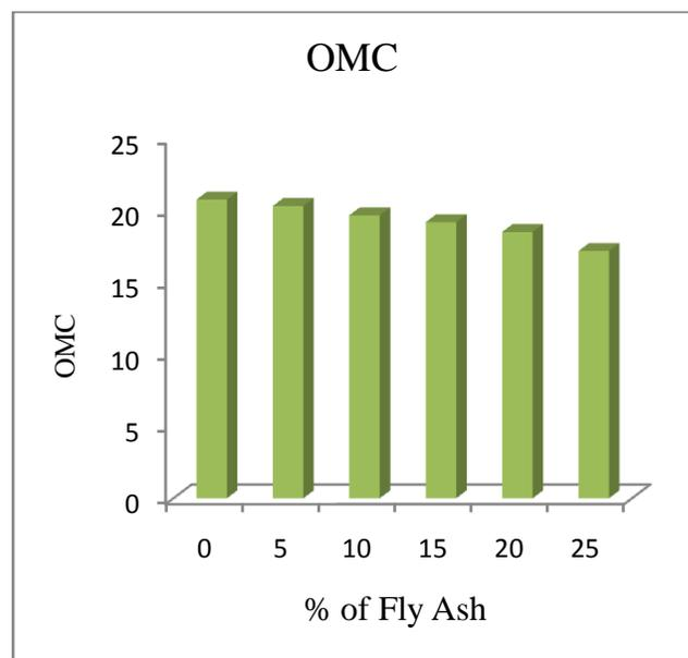
**Figure.1. Effect of Fly Ash on OMC**
