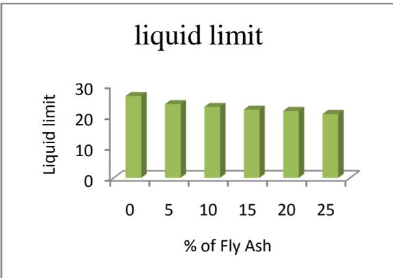
**Figure. 3. Effect of Fly Ash on liquid limit**
