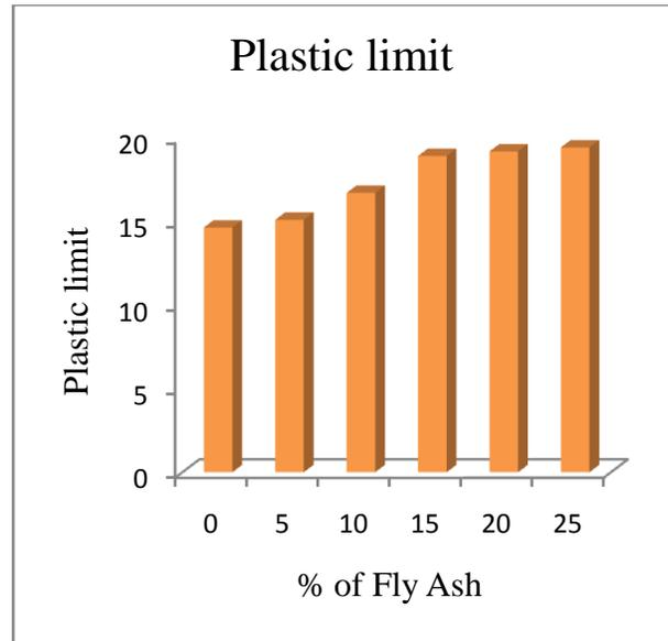
**Figure.4. Effect of Fly Ash on plastic limit**
