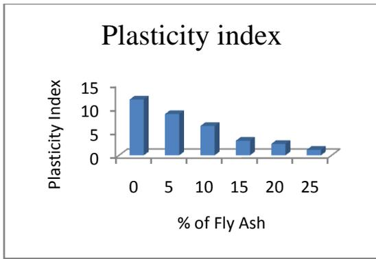
Figure. 5. Effect of Fly Ash on plasticity Index
