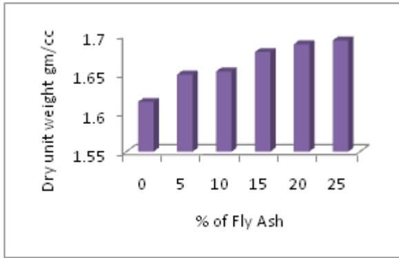
**Figure.2. Effect of Fly Ash on MDD**
