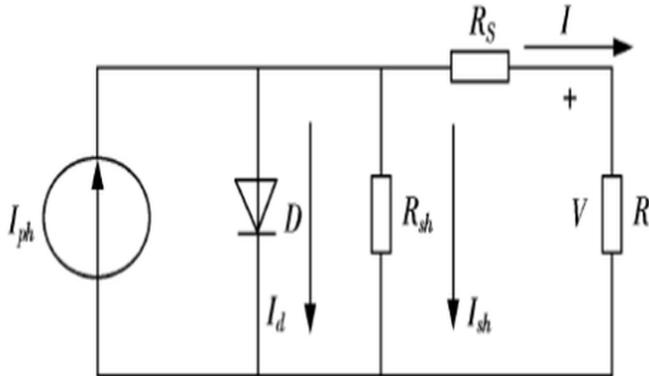
The well-known single diode electrical equivalent circuit for a PV cell is shown in fig 1.
