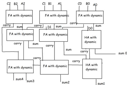
**Figure.7. Carry save adder with dynamic block**
