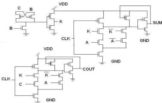
Figure.2. Full adder with Domino logic
