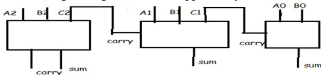
Figure.3. Ripple Carry Adder block diagram
