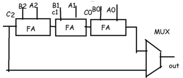
Figure.4. Carry Bypass Adder
