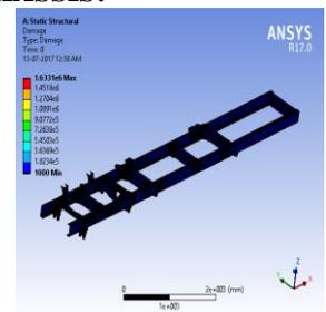
Figure. 12. Damage for AISI A514 GRADE B
