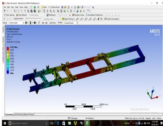
Figure.6. Displacement pattern for AISI 4130 Steel alloy
