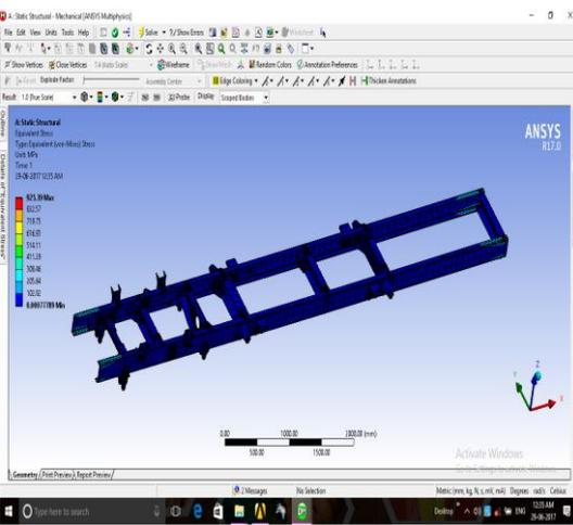
Figure.5. Stress distribution for AISI 4130 steel alloy
