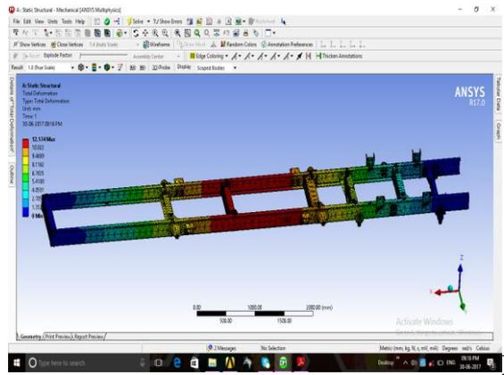
Figure.8. Displacement distribution of A790M GRADE 345W alloy steel
