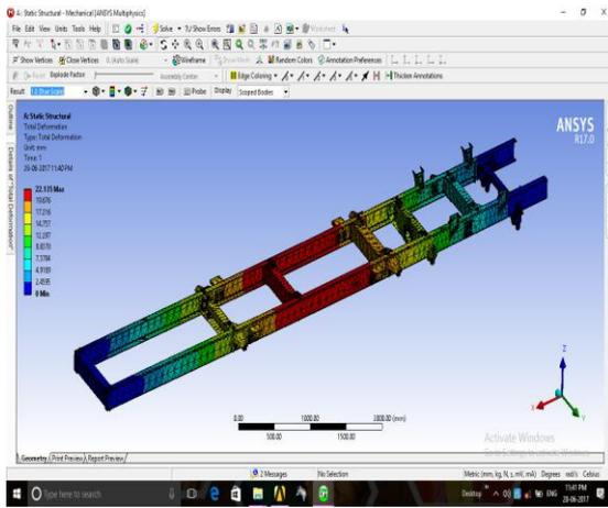
Figure.4. Displacement pattern for grey cast iron
