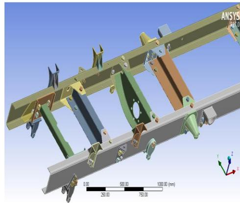
**Figure.1. Assembly Design of chassis**
