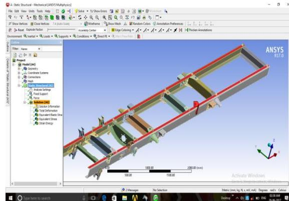
**Figure.2. Boundary conditions of chassis**
