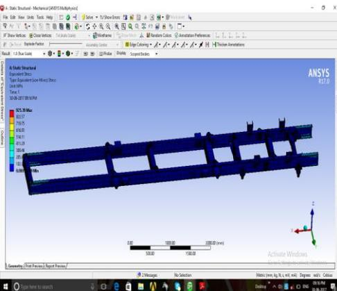
Figure.7. Stress distribution of A790M GRADE 345W alloy steel
