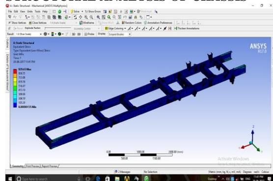
**Figure.3. Stress distribution for grey cast iron**
