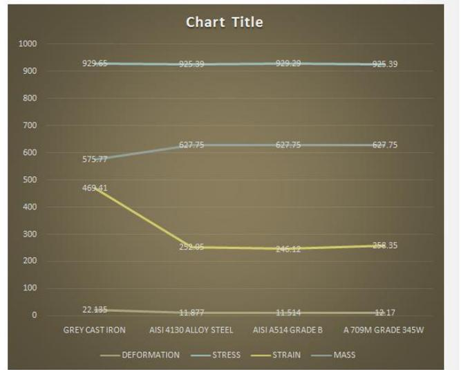
Graph.1. Comparative analysis of structural steel chassis and other alloy steels
