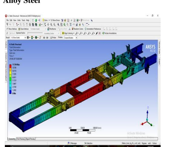
Figure.10. Displacement distribution for AISI A514 GRADE B Alloy Steel
