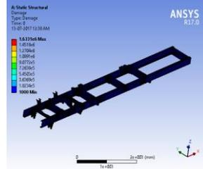
Figure.16. Damage for A 709M GRADE 345W
