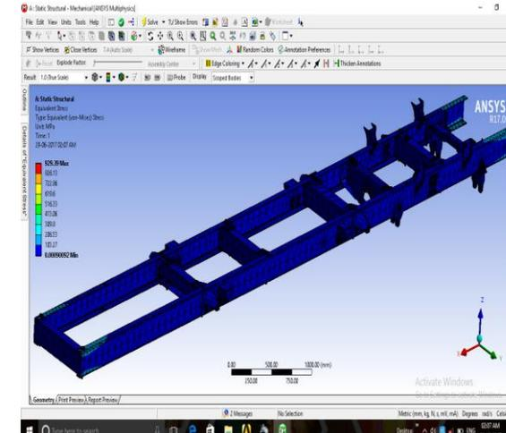
Figure.9. Stress distribution for AISI A514 GRADE B Alloy Steel
