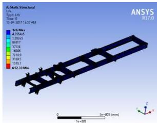
Figure.15. Life for A 709M GRADE 345W
