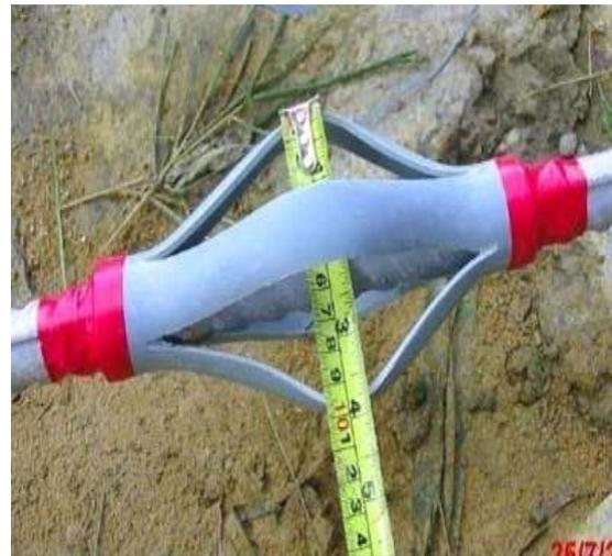
Figure.3. Typical Centralizers
