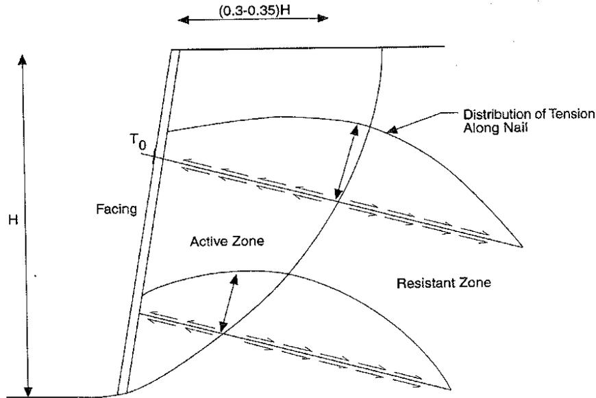
Figure.1. Conceptual soils nail behavior (Byrne et al., 1998)
