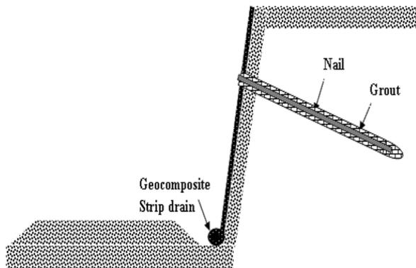
Figure.8. Nail Installation and Grouting (Byrne *et al.*, 1998)
