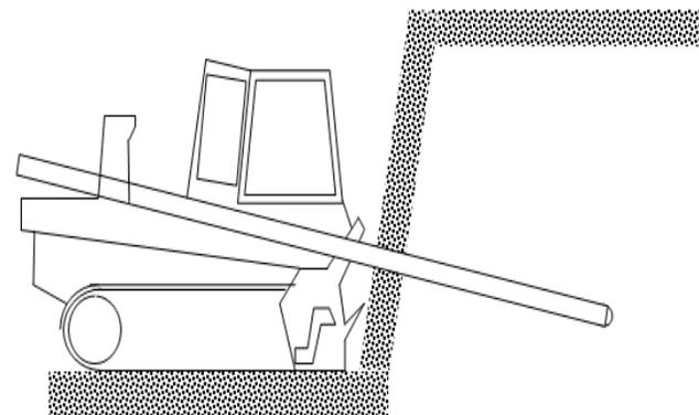
Figure.7. Drilling Nail Holes (Byrne *et al.*, 1998)
