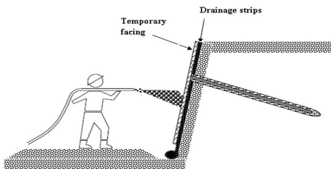
Figure.9. Construction of Temporary Shotcrete Facing (Byrne *et al.*, 1998)
