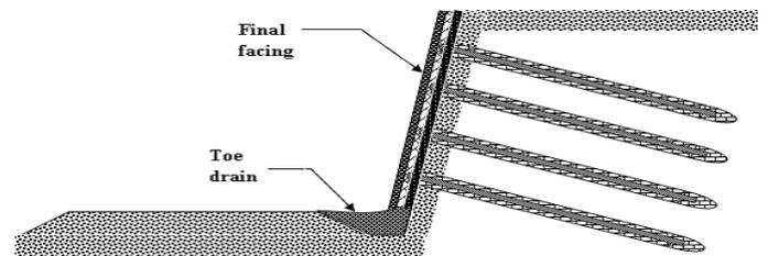
Figure.11. Construction of Permanent Facing (Byrne *et al.*, 1998)
