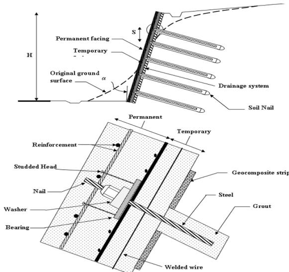
Figure.5. Typical cross-section of a drilled soil nail wall (Byrne *et al.*, 1998)
