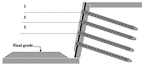
Figure.10. Construction of Subsequent Levels (Byrne *et al.*, 1998)
