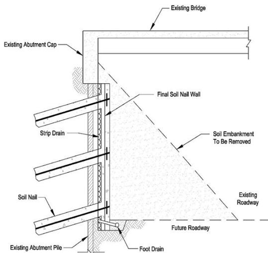
Figure.13. Road Widening under Existing Bridge Abutments (lazarte *et al.*, 2015)
