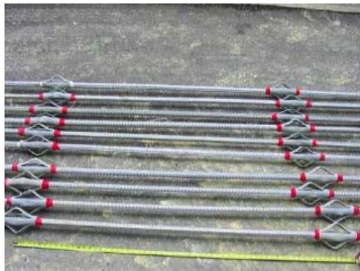
Figure.2. Soil nails reinforcement Bars
