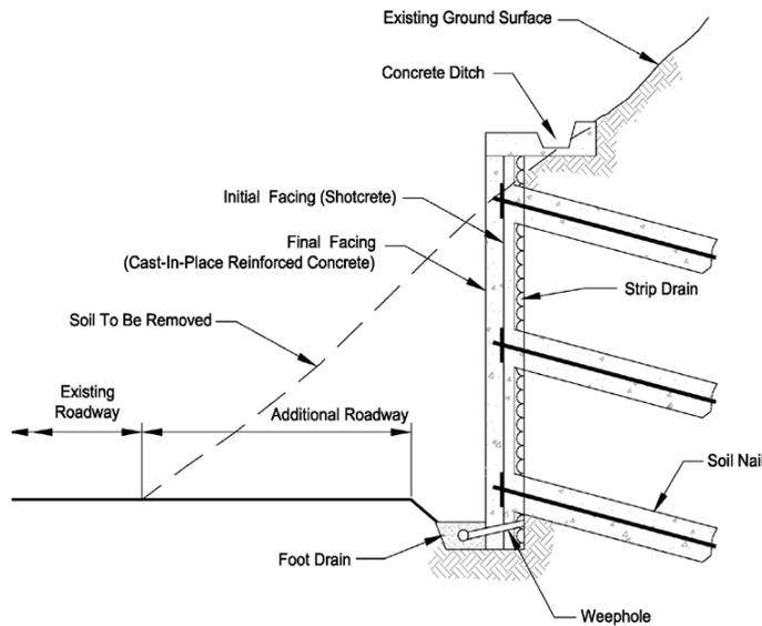
Figure. 12. Roadway Cuts (lazarte *et al.*, 2015)
