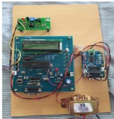
The transformer is used to convert 230 KV to 12 V to give power supply to the kit. The bridge rectifier converts alternating voltage to direct voltage and filter is used to remove the ripples. The heart beat sensor, temperature sensor and respiratory sensor is connected to the PIC microcontroller. The LCD display is connected to display the values of the temperature, heartbeat and respiration. The Zigbee module is used for wireless transmission of the values to the AR headset receiver.
