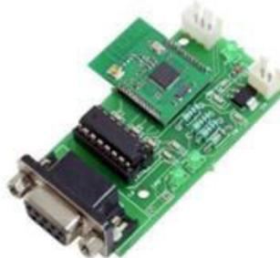
**Figure .7. Zigbee module**
