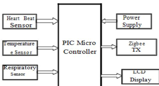
Figure.1. Transmitter section
