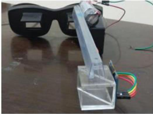
The receiver section consists of a Dc battery, Zigbee receiver module and OLED display. The Zigbee receiver receives the values that are transmitted and displays in OLED display connected to it. Through the wearable glass the information such as the temperature, breathing and heart beat rate is displayed by using a prism. The prism is used for enhancing the display of characters.
