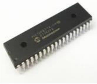
**Figure.3. PIC Microcontroller 16F877A**
