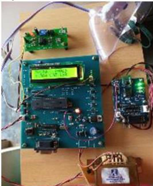
The output gives the temperature ( T ),Heart beat rate ( H ) and Breathing rate ( R ) of a normal healthy person. In case of an abnormal condition it gives an alert to the doctor by displaying the message 'ALERT'. The range of abnormal value for temperature is above 40°C. The range of abnormal value for heart beat is above 75 beats per minute (bpm) and for breathing rate is above 100 breaths per minute (bpm).
